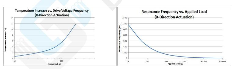
• These temperature rises were measured after applying a sine-wave drive voltage ranging from 0 to 200V at the specified frequency for 10 minutes.
