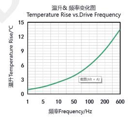
These temperature rises were measured after applying a sine-wave drive voltage ranging from 0 to 100V at the specified frequency for 10 minutes.
