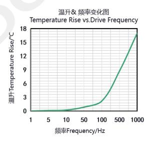
These temperature rises were measured after applying a sine-wave drive voltage ranging from 0 to 150V at the specified frequency for 10 minutes.
