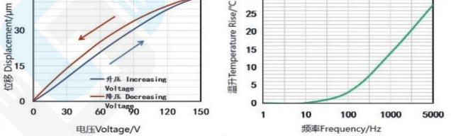
• These temperature rises were measured after applying a sine-wave drive voltage ranging from 0 to 150V at the specified frequency for 10 minutes.
