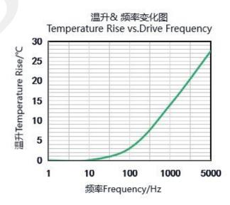
• These temperature rises were measured after applying a sine-wave drive voltage ranging from 0 to 120V at the specified frequency for 10 minutes.
